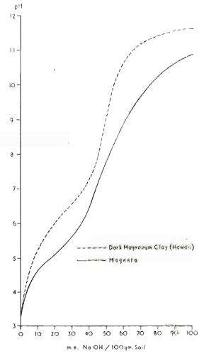
Fig. 13. Titration curve of the dark magnesium clay of Hawaii and that of a local soil of the same nature.
