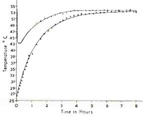
Fig. 22. Temperatures inside air oven (dots) and at the centre of a cutting (crosses) during an 8 hour heat treatment.
