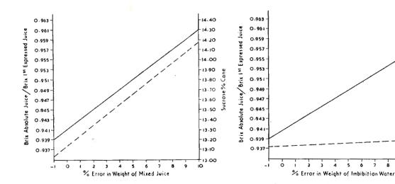
Fig. 29. Influence of weight of mixed juice on ratio BA/B1 (plain line) and on sucrose content (broken line).
