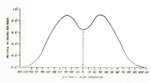
Fig. 26. Distribution of water at varying distances from rainer.
