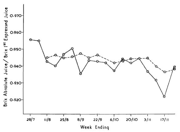
Fig. 28. Weekly variations in the ratio BA/B1 for factory A (broken line) and for factory B (plain line).
