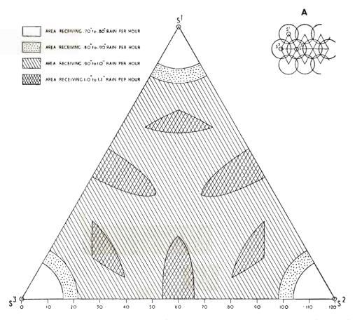
Fig. 27. Distribution of water from sprinklers S1, S2, S3 when arranged in the conventional patern shown at A.
