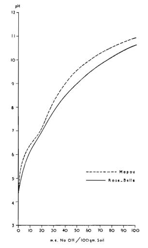
Fig. 14. Titration curves of two immature local soils.
